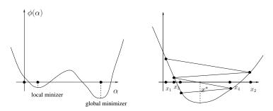
The search algorithm should allow step length  $\alpha$  large enough to find the global minimizer, but also small enough to reduce the oscillations around the minimizer.
