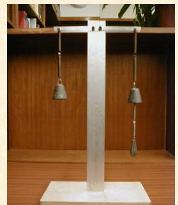
b). A model of a SDOF and a TDOF systems
