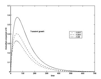
FIG. 1. Linear case: the azimuthal component  $B_{\varphi}$  as a function of time  $[B_{\varphi}(0)=0]$  for g=1,  $\delta=10^{-4}$ , and  $\varepsilon=2\times10^{-2}$  and different initial values of  $B_r$ , -0.017, -0.021, and -0.03.
