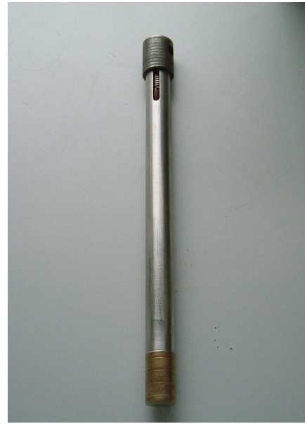
Figure 2.3 25mm diameter steel piston rod
