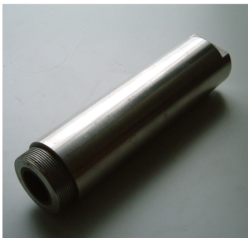
Figure 2.5 25mm diameter cylindrical steel barrel to be used as larger reservoir
