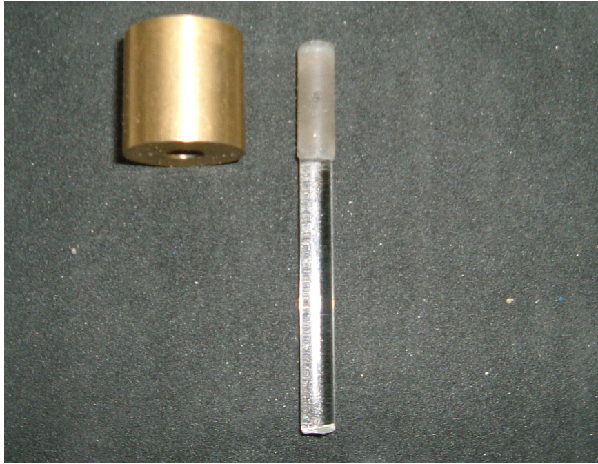
Figure 2.10 Failed prototype for bonding glass to brass using silicone sealant
