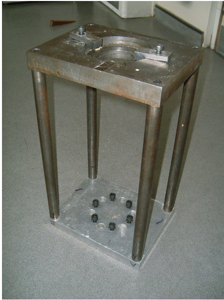
Figure 2.2 Steel test frame with base plate and top plate
