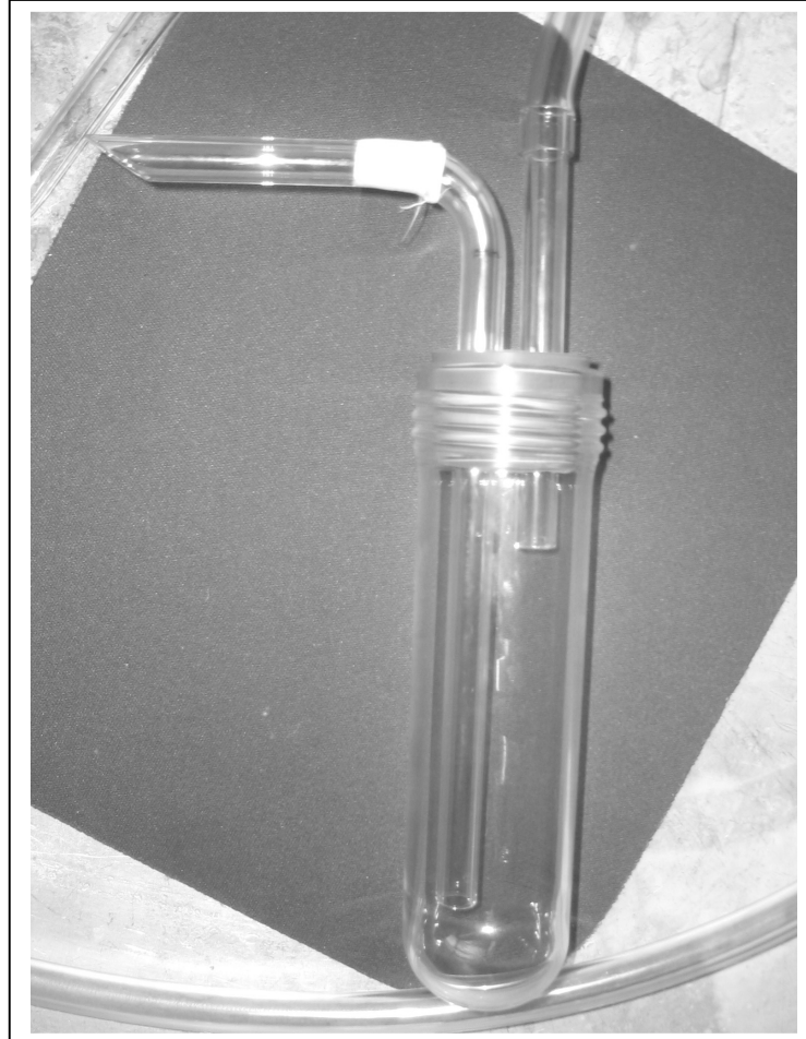
Figure 3.4: A photograph of the foam sampling tool.
