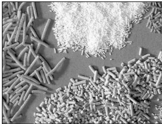
Figure 1.3 Selection of granules produced with Fuji Paudal extruders Reproduced from Fuji Paudal promotional brochure. No scale was given.
