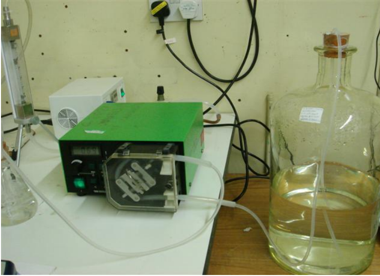
Figure 19: Pump was connected through a plastic tube to the large vessel and also the inverted J-shaped foam fractionation column
