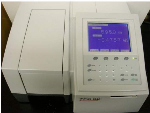
Figure 18: UV-VIS Spectrophotometer. This device is used to measure the absorbance of samples collected from foam fractionation process. For example, in this case the absorbance is measured as -0.4757 ABS at 595nm wavelength.
