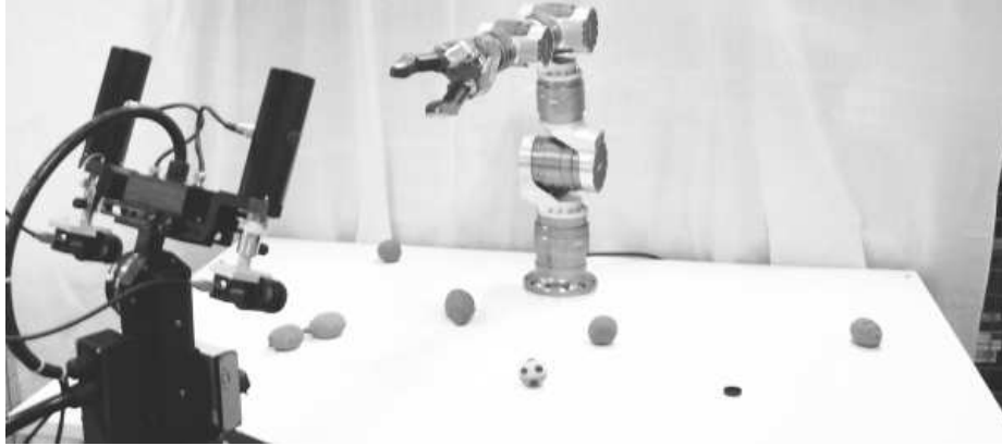
Fig. 1. Robotic arm and manipulator system mounted on a table and the active vision system, scanning the scenario with two cameras and a SCAMP vision system.
