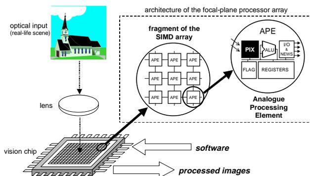
Fig.1. A programmable SIMD focal-plane processor array
