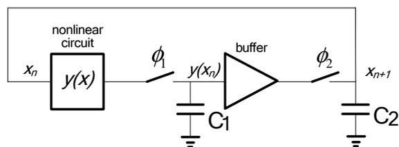
Fig.1. Discrete-time chaos generator circuit
