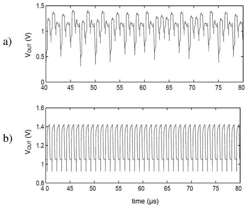
Fig.6. Simulated voltages at the map circuit output; (a) chaotic signal for  $V_C=1.6\text{ V}$ ; (b) periodic signal for  $V_C=0.6\text{ V}$ .
