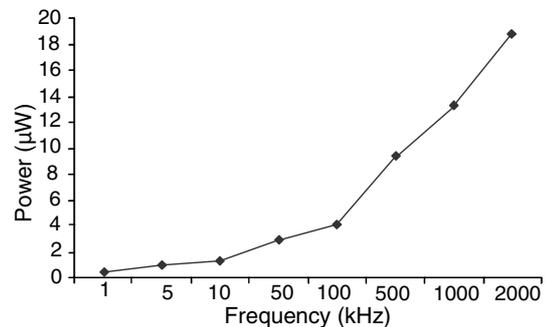
Fig.7. Power consumption of the chaos generator as a function of operating frequency
