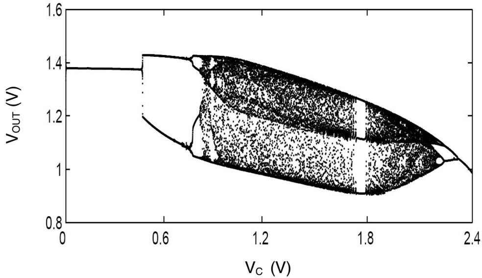
Fig.5. Simulated bifurcation diagram of the proposed chaos generator
