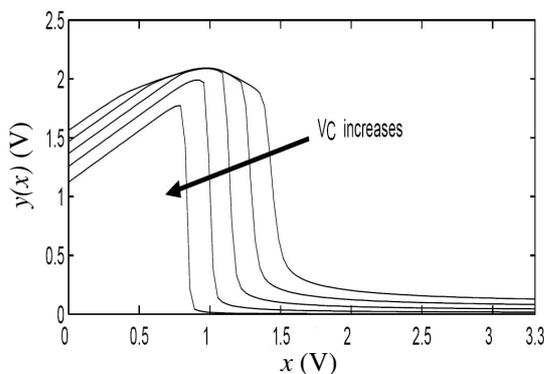
Fig.3. The DC characteristics of the three-transistor map circuit
