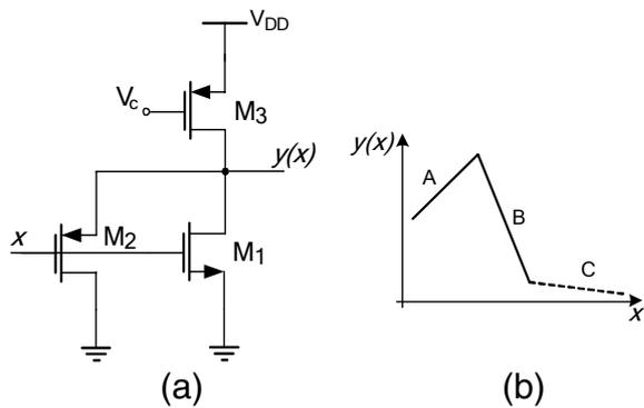
Fig.2. (a) three-transistor map circuit (b) a “tent-like” map transfer characteristic
