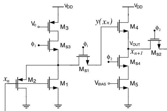
Fig.4. Circuit diagram of the proposed chaos generator
