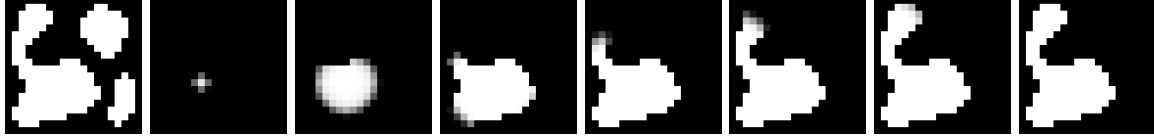
Figure 5. Geodesic Reconstruction. Input image (left) and state captured at 0.5 ns intervals
