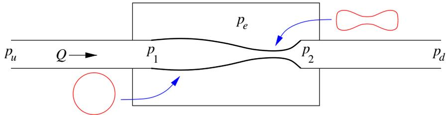
**Fig. 1.** The Starling Resistor. A flux  $Q$  is driven from left to right by a pressure drop between inlet and outlet (at pressures  $p_u$  and  $p_d$  respectively). The collapsible segment of tube is subject to external pressure  $p_e$  and may buckle to a non-axisymmetric cross-section when collapsed, as indicated.
