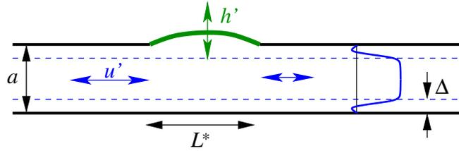
**Fig. 3.** Sloshing in a 2D channel: the membrane length  $L^*$  exceeds the channel width  $a$ ; transverse wall motions of amplitude  $h'$  drive axial flows of magnitude  $u'$ ; at high frequencies, Stokes layers of width  $\Delta$  are thin compared to the channel width.
