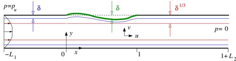
**Fig. 4.** The asymptotic structure of sloshing flows in a 2D channel. Stokes layers have dimensionless thickness  $\delta \ll 1$ ; membrane displacements are  $O(\delta)$ ; steady streaming boundary layers have thickness  $\delta^{1/3}$ .
