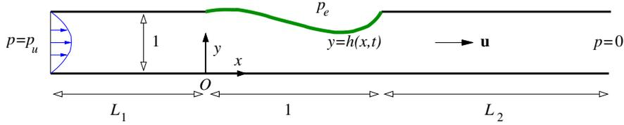
**Fig. 2.** The 2D analogue of the Starling Resistor. Flow is driven by a fixed pressure drop  $p_u$  through a finite-length channel, one wall of which contains a flexible membrane under external pressure  $p_e(x)$ . Distances  $x$  and  $y$  along and across the channel are scaled on the length of the flexible segment and the channel width.
