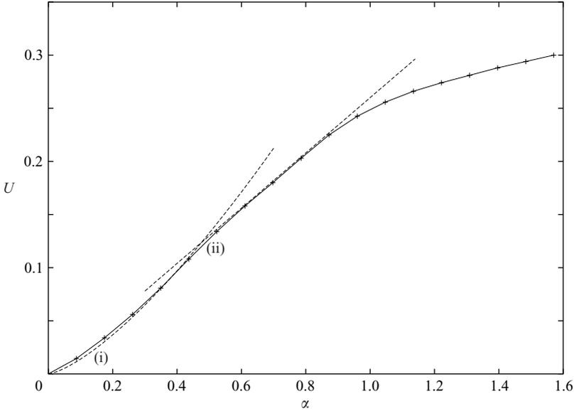
FIGURE 10. Symbols show drop speed with  $B = 2.023$ ,  $\lambda = 1$ , as a function of channel inclination, taken from DeBisschop *et al.* (2002). Dotted lines show (i)  $U = 0.4\alpha^{3/2}$  and (ii)  $U = 0.3\alpha$ .
