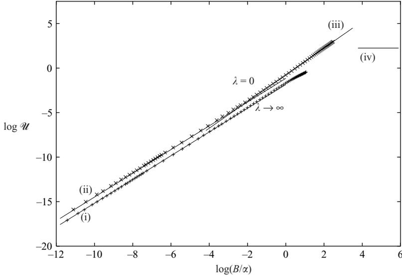
FIGURE 7. Numerical and asymptotic results for the drop speed for sliding ( $\lambda \rightarrow \infty$ ) and slipping ( $\lambda = 0$ ). The four solid lines are the asymptotes (i)  $\frac{4}{3} \log(B/\alpha) - \frac{8}{3} \log 2$ ; (ii)  $\frac{4}{3} \log(B/\alpha) - \frac{5}{3} \log 2$ ; (iii)  $\frac{3}{2} \log(B/\alpha) + \log(0.497)$ ; (iv)  $\log(9.57)$ .
