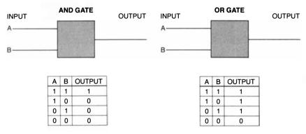
CONVENTIONAL LOGIC GATES dissipate energy because they discard information. For example, if the output of an *and* gate is 0, there is no way to deduce what the input was.
