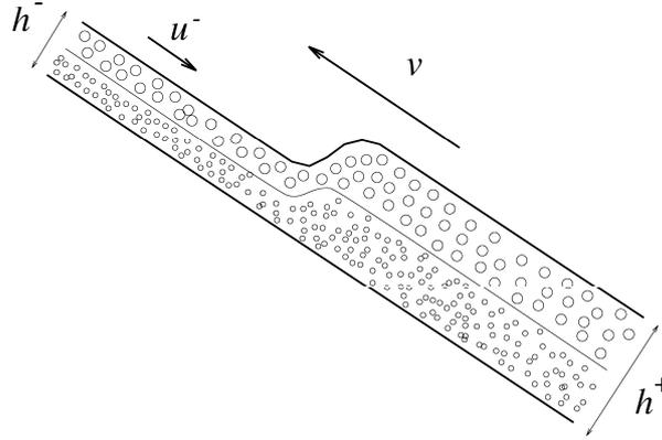
*Figure 2.* The photograph shows the propagation of a granular shock on the free surface of a stratified stationary deposit. The flow in the two layer shear band is brought to rest, as the jump propagates upslope, freezing the particle size distribution into the material to form a stripe.
