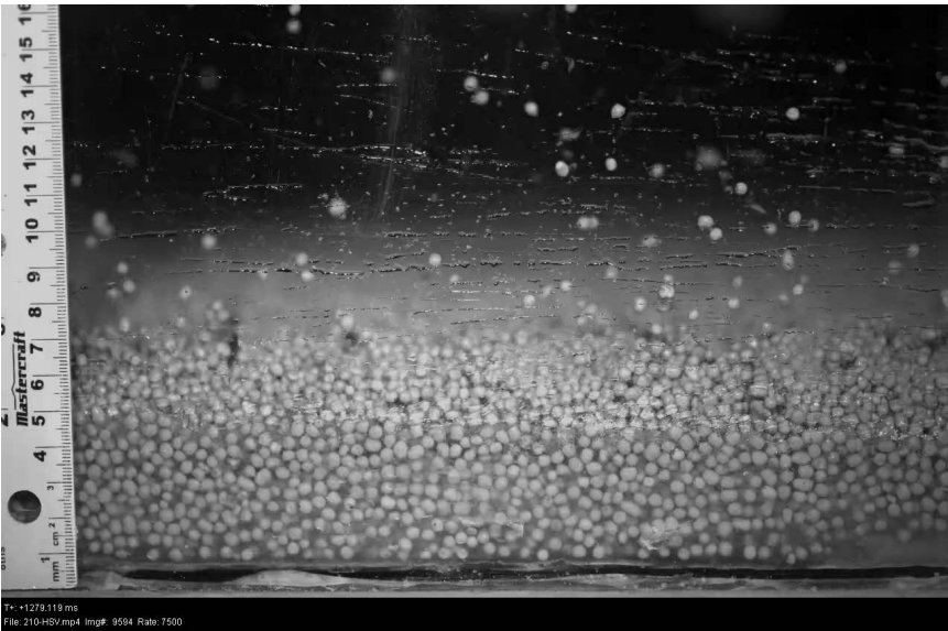
Figure 3. Taylor-Noonan et al. 's (2022) high-speed movie images of the (a) dry and (b) wet flow experiments 0.5 m upstream of the slope break, 0.94 s after the initial front arrival and for initial volumes V_{ini} = 0.8 \text{ m}^3 . Movies 3 and 4 in the online supplementary material show the complete high-speed movie sequences, which are very instructive. All of Taylor-Noonan et al. 's (2022) high-speed camera data is available from https://doi.org/10.5683/SP3/IZCUFY .
