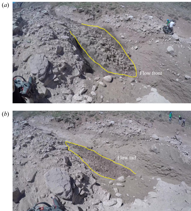
Figure 1. Debris flow on 27 January 2015 in Aconcagua Park, Mendoza, Argentina (copyright Julian Insarralde via ViralHog). (a) A large amplitude dry bouldery flow front propagates down a channel at approximately 6 \text{ m s}^{-1} , forcing hikers to scramble to safety. (b) Eighteen seconds later, the height of the flow has reduced, there are no surface boulders and the flow is much more watery. Movie 1 in the online supplementary material shows that the main pulse is followed by a series of bouldery surges, 40, 71 and 160 seconds after the arrival of the main front, which are interspersed by lower amplitude watery sections.
