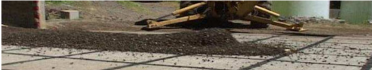
FIGURE 1. Experimental debris-flow deposit at the United States Geological Survey (USGS) flow flume, Oregon, USA, August 2008 (Logan & Iverson 2013). The back of the flow has a constant height, while the front shows evidence of a bulbous head; the flow is higher near the front than at the back of the flow. Picture courtesy of USGS.
