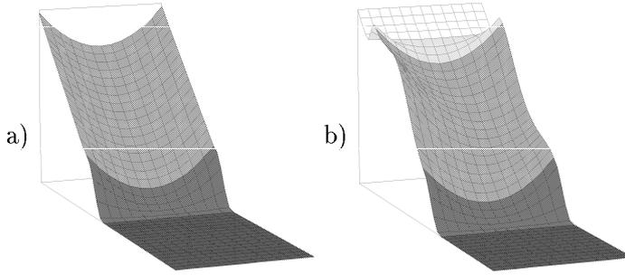
*Figure 2.* The basal chute geometry used in the experiments and numerical computations: a) symmetric parabolic chute (V02), b) the snaking valley chute (ISO3). The shading highlights the different zones in the respective chutes.
