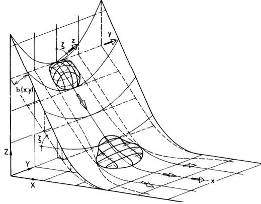
*Figure 1.* The simple curvilinear coordinate system  $Oxyz$  consists of an inclined plane connected to a horizontal plane by a smooth transition. The local inclination angle of the curvilinear surface  $z = 0$  (dashed lines) is  $\zeta$ . The actual basal topography  $z = b(x, y)$  (solid lines) is superposed to top of the  $z = 0$  curvilinear surface.
