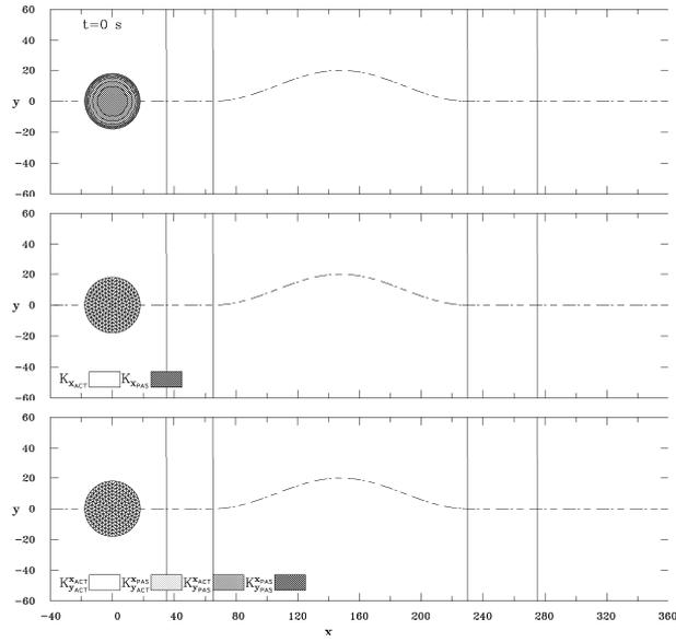
*Figure 8.* The same as Fig. 3 except for experiment ISO3. Initially the granular material is released on a  $40^\circ$  inclined plane. The lines at  $x = 35, 65, 230, 275$  cm indicate the position of the transition zones between the inclined plane, the sinusoidal snaking valley and the horizontal plane. The dashed line shows the position of the 'Talweg'.
