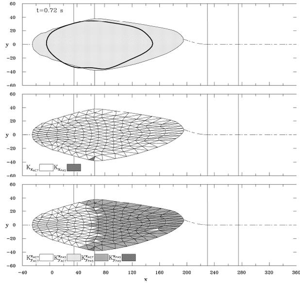
*Figure 9.* The same as Fig. 8. The thick line in the top panel indicates the experimentally determined position of the avalanche edge.
