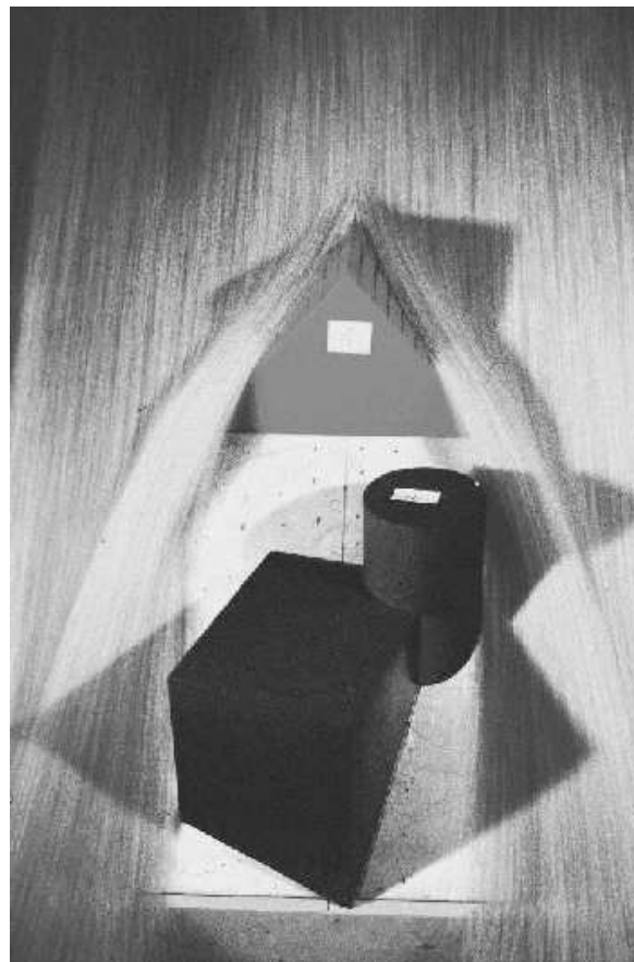
Figure 5. An oblique shock is also shed on either side of an avalanche defence structure (grey), which can be clearly seen from the streamlines. The avalanche flows from the top to the bottom of the image. On the lee side of the defence a granular vacuum is formed (white) which protects the structure below (black) from contact with the avalanche
