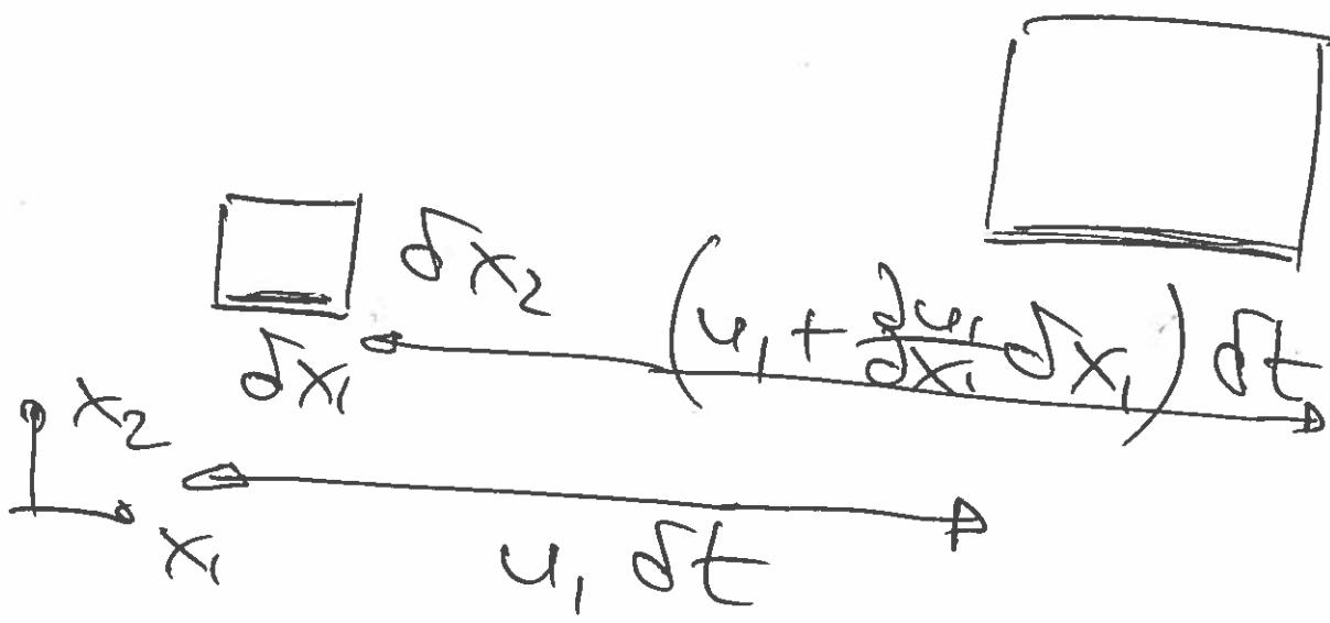
$$\text{Strain} = \frac{\text{length - old length}}{\text{old length}}$$
