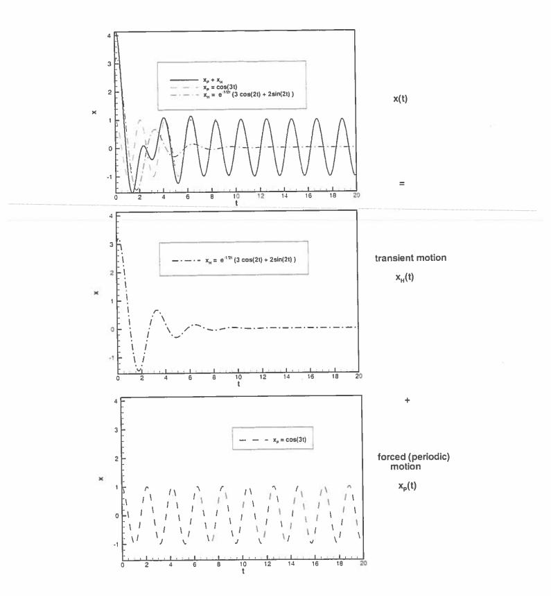
Figure 5: The displacement of a harmonically-forced, damped mechanical oscillator comprises the periodic (forced) solution  $x_P(t)$  and the transient solution  $x_H(t)$ .
