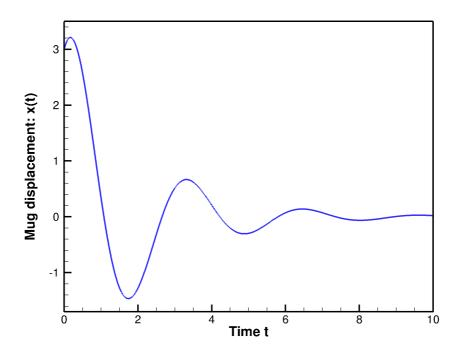
• Damped oscillation with certain characteristic frequency – the system's "eigen" frequency.
