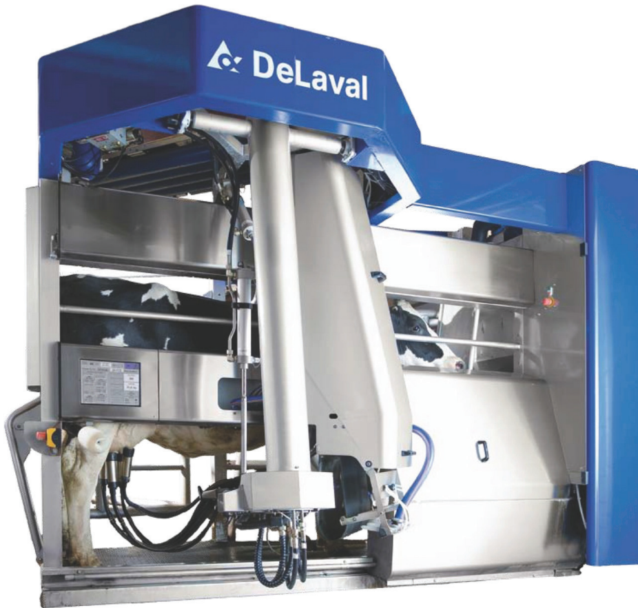
Figure 4.5 A typical automatic milking system. The cow is barely visible inside, although most animals are easily trained to accept the machine and the robotic processes. Courtesy of DeLaval A/S.
