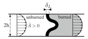
FIG. 2. Premixed flame (with thickness  $\delta_L$ ) propagating in a channel of height 2*h* against a flow of amplitude  $\hat{A}$ . The main parameter is  $\epsilon = h/\delta_L$ .
