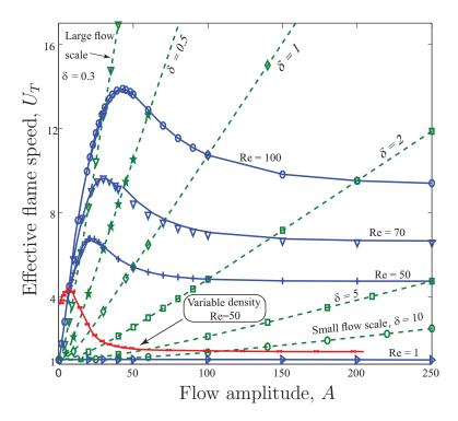
FIG. 3. Propagation speed  $U_T$  versus the flow amplitude A of a Poiseuille flow for fixed values of Re (solid curves) or fixed values of  $\delta \equiv \epsilon^{-1}$  (dashed curves). Results of constant density numerical calculations are shown, except for the solid red curve labeled "Variable density," which shows variable density calculations for fixed Re = 50.
