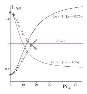
FIG. 4. Effective Lewis number  $\text{Le}_{\text{eff}}$  versus the scaled Péclet number  $\text{Pe}_s \equiv \text{Pe}(1 - \alpha)$  for fixed values of Le. Solid lines denote analytical results from Eq. (23). Circles and squares denote numerical results for Le = 0.75 and Le = 1.25, respectively, computed in the constant density approximation (where  $\text{Pe}_s = \text{Pe}$ ) and for fixed  $\epsilon = 0.01$ .
