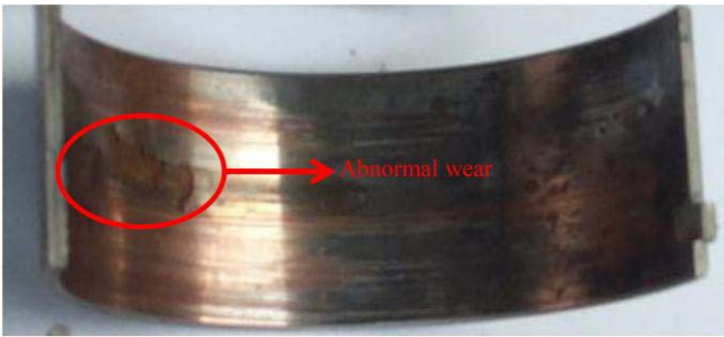
Fig. 9. Abnormal wear in the bush of main bearing.
