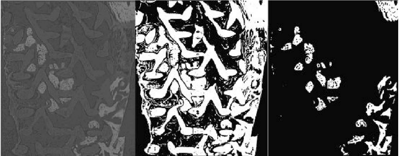
Fig. 6. Slice of PCL graft tomogram illustrating segmentation; grey level image (left); bone and scaffold (middle); and bone (right).
