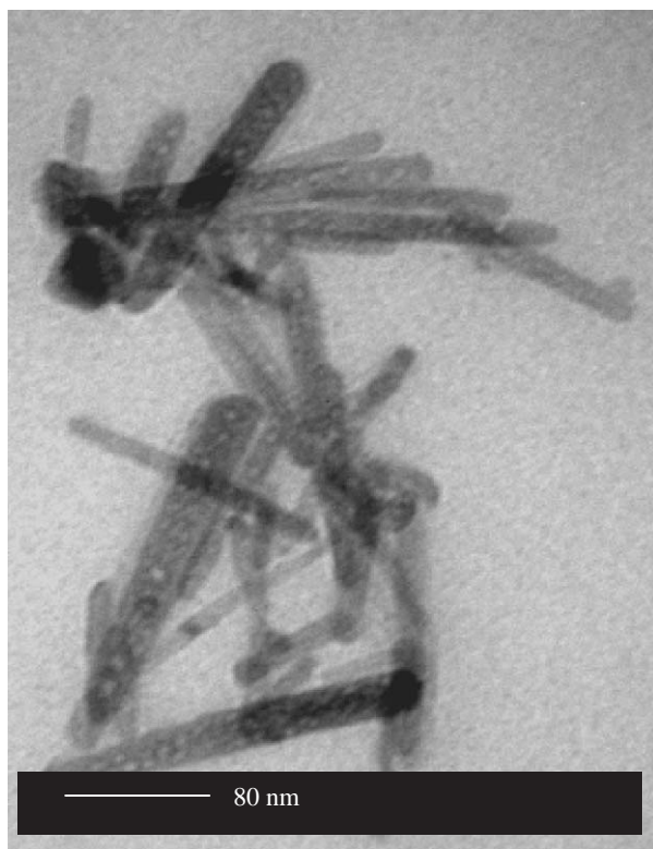
Fig. 2. TEM micrograph of hydroxyapatite nanofibers prepared by a biomimetic method.
