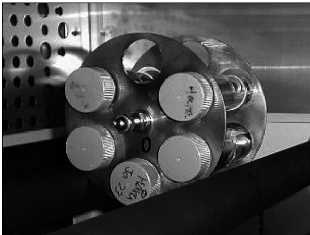
Fig. 2. Original designed vessel holder placed on roller device (6 RPM) in an incubator (5% CO_2 in air, 37 °C, fully humidified).
