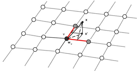
Fig. 1. Local linear projection.  $\mathbf{x}$ : data point,  $v$ : winning node, and  $\mathbf{x}'$ : the projected point on the map.
