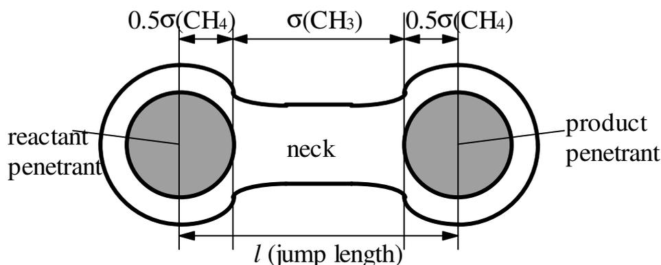
**Figure 5.1:** Sketch showing how the jump length,  $l$ , is constructed, given the assumed geometry of the cavities and neck.
