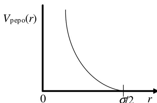
**Figure 5.7:** Qualitative sketch of  $V_{\text{papo}}(r)$ , the energy for the penetrant to push through the neck.  $\sigma$  is approximately the Lennard-Jones diameter of the penetrant,  $\sigma_p$ .
