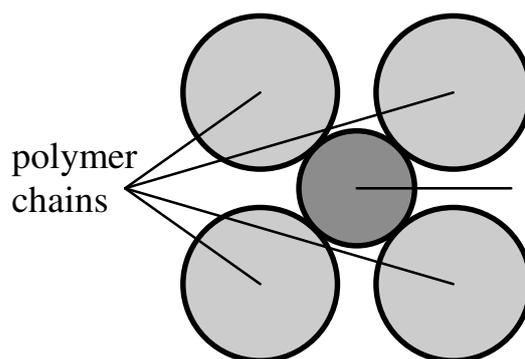
**Figure 2.2:** Sketch illustrating position of penetrant in relation to polymer chains. The penetrant moves perpendicular to the page parallel to the polymer chains.
