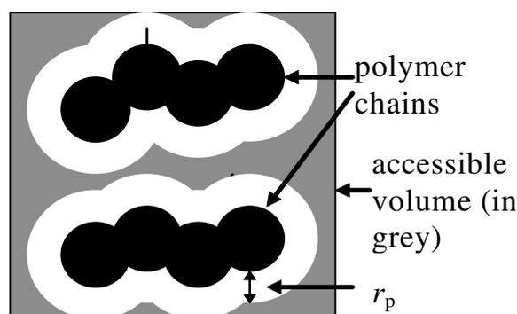
**Figure 4.3:** Illustration of regions of accessible volume for a penetrant with hard sphere radius  $r_p$ .
