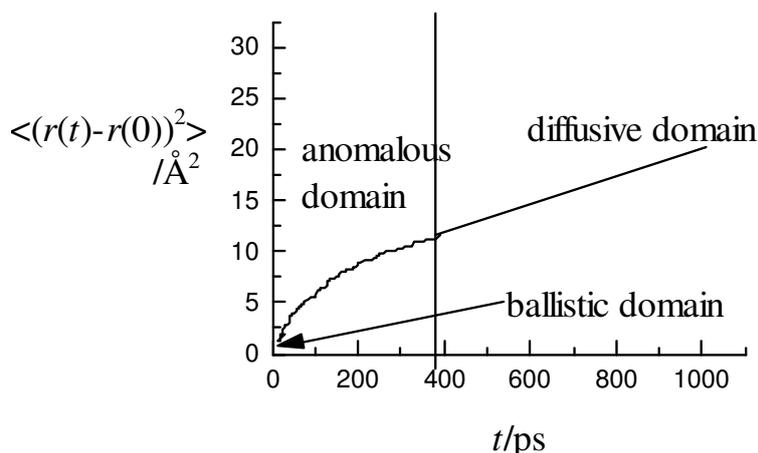
**Figure 4.1:** Typical plot of  $\langle (r(t)-r(0))^2 \rangle$  versus time for diffusing penetrants, showing the three time domains. The ballistic domain shows up as a quick rise in displacement at very short times.
