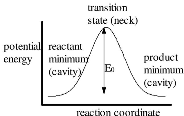
**Figure 4.2:** Potential energy along the reaction coordinate, the minimum energy path between reactant and product minima. The transition state is taken as the maximum on this path.
