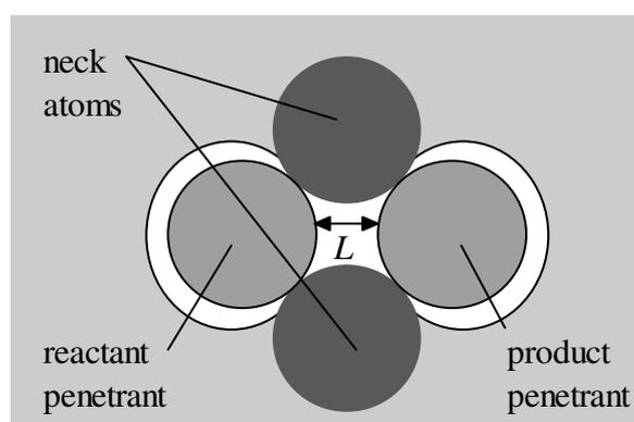
**Figure 5.2:** A possible neck structure such that  $L$  is less than the diameter of the neck atoms.
