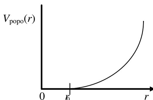
**Figure 5.5:** Qualitative sketch of  $V_{\text{popo}}(r)$ , the energy required to form a neck of radius  $r$ .  $r_0$  is the radius of the pre-existing neck in the reactant state.
