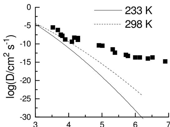
**Figure 5.12:** Prediction of the model of how  $D$  varies with penetrant Lennard-Jones diameter at  $T = 233$  and  $298$  K. The points are experimental data for various penetrants in PVC (Koros *et al.*, 1988)
