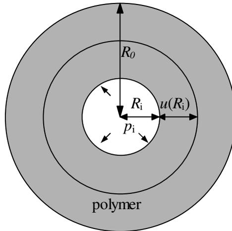
**Figure D.1:** Cross-section of the hollow cylindrical polymer pipe.  $R_0$  and  $R_i$  are outer and inner radii.  $p_i$  is the pressure applied to the inner surface.
