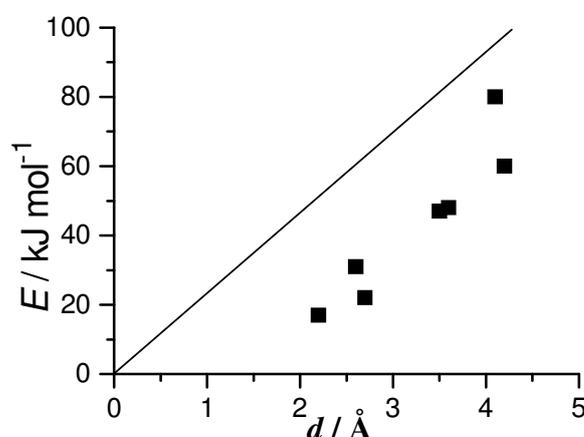
**Figure 2.3:** Comparison with experiment (dots; Meares, 1954,1957) of the theoretical apparent activation energies,  $E_{app}$ , (solid line) versus penetrant diameter,  $d$ , for glassy polyvinyl acetate (Pace and Datyner, 1977c). Shifting the curve right by 1.5 nm would produce agreement between the two.
