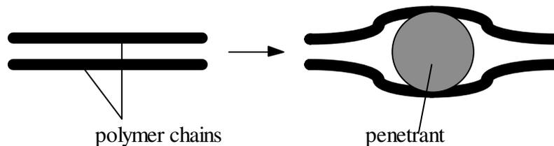
**Figure 2.1:** Sketch illustrating the assumed activated mechanism of Brandt, in which two polymer chains move apart to allow a penetrant to fit between them.
