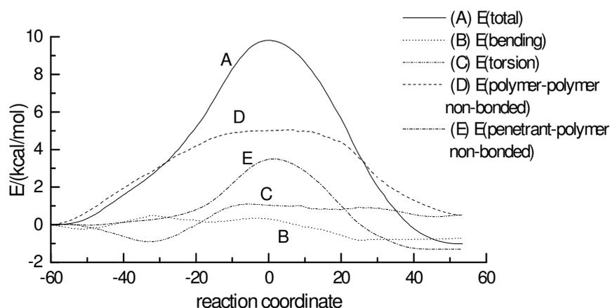
**Figure 5.3:** The energy profile along the reaction coordinate for jump number 4. Shown also are the changes in the individual energy contributions (bends, torsions, polymer-polymer non-bonded, penetrant-polymer non-bonded). Note that the energy is in kcal/mol.
