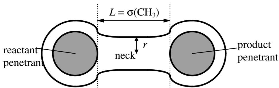
**Figure 5.4:** Diagram showing the assumed structure of the neck connecting reactant and product cavities as a cylinder, with radius,  $r$ , and length  $\sigma(\text{CH}_3)$ .
