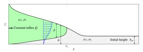
FIGURE 1. (Colour online) Schematic illustration of the set-up and the definition of variables. The fluid properties give rise to a viscosity ratio  $m = \mu_2/\mu_1$  and a relative density difference  $\varepsilon = \rho_2/\rho_1 - 1$ .
