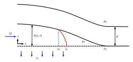
FIGURE 1. (Colour online) Schematic diagram of a current propagating below an elastic sheet with leakage. The figure indicates the coordinate system and illustrates the various dimensional variables. The red line denotes the profile of the current in the region  $x_F < x < l_d$ . We consider that the fluid spreads laterally from the source in both the +x and -x directions; however, we exploit the mirror symmetry of the system about the injection point and consider only the +x direction.
