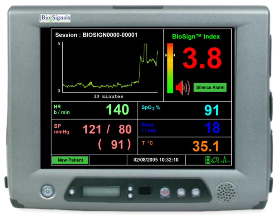
Figure 3: The output of the data fusion algorithm, as displayed on bedside tablet PCs
