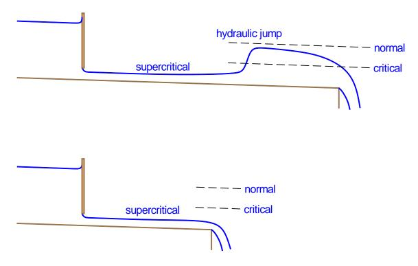
(c) As the channel shortens, the depth change across the hydraulic jump diminishes. The boundary between the two possible flow behaviours occurs when the supercritical GVF just reaches critical depth at the overfall (i.e. the limiting depth change across the hydraulic jump is zero).
