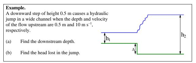
(a) The downstream depth can be deduced from the momentum principle if the reaction force from the step is known. The approximation is that this is the same as would occur if it were in equilibrium with a hydrostatic pressure distribution here.
