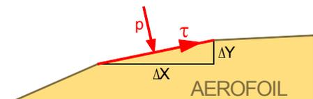
Show how to use this data to produce drag and lift coefficients for the aerofoil, separating values for pressure, viscous and total forces. Confirm that the total drag and lift coefficients yield the values reported by the program and comment on the relative size of the pressure and friction contributions to lift and drag.
