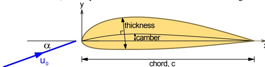
The aerofoil section may be *either* an analytical profile for the NACA 4-digit series:
