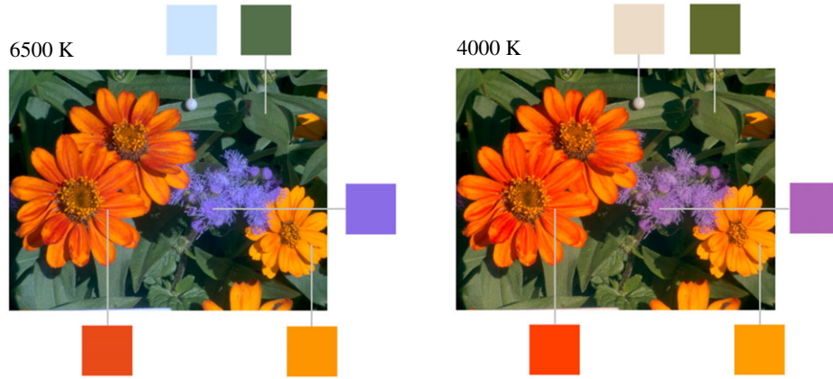
Figure 1. Colour images of a scene under different simulated daylight. The images are rendered as sRGB images [13] from a hyperspectral reflectance image [14] with a daylight illuminant of correlated colour temperature of 6500 K in the left panel and 4000 K in the right panel. The square patches are enlarged copies of the indicated pixels. (Online version in colour.)
