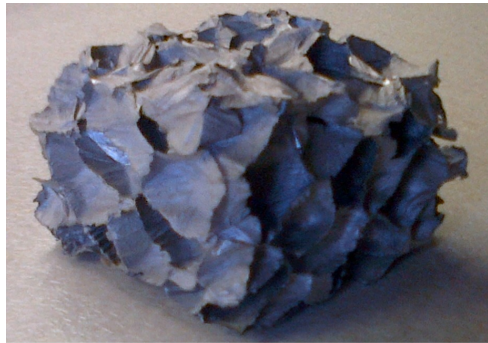
Figure 2: Aluminium foam with a narrow Gaussian-like distribution of void sizes of around 1cm diameter partially wrapped in fragmented metallic shells, used as crushable buffers inside vehicle bodies. The cosmological void distribution is by contrast gamma-like with a long tail [8], interspersed with 60% of galaxies in large-scale sheets, 20% in rich filaments and 20% in sparse filaments [12]. Such 3D stochastic porous materials can both be studied by tomographic methods, albeit at different scales by different technologies, yielding sequences of 2D stochastic texture images.
