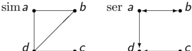
In a step trace monoid, since  $\text{ser} \cap \text{ser}^{-1} \cap \text{inl} = \emptyset$ , we can put  $\text{ser}$  &  $\text{inl}$  on the same graph, with  $\text{inl}$  edge undirected.
