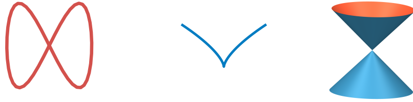
FIGURE B.5 None of these sets are submanifolds: the figure–8, the semicubical parabola (cusp) and the cone; each has one singular point.
