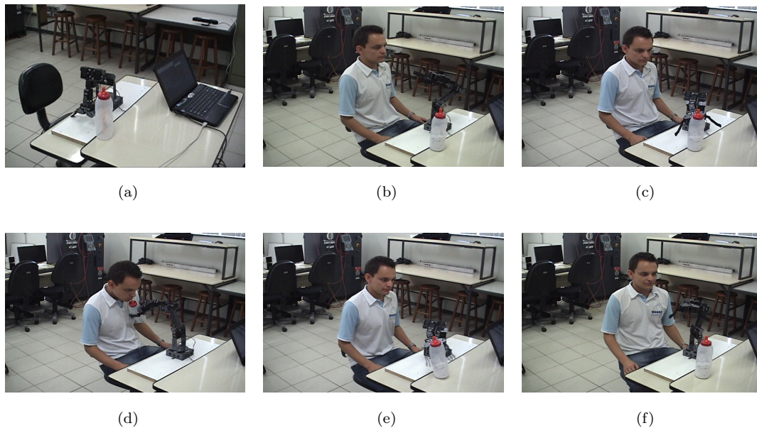
Figure 10: Example of one sequence for the task execution: (a) the environment of the task, (b) the robot at its initial pose, (c) the bottle reaching, (d) the drink serving, (e) the robot returning the bottle to the table, and (f) the robot returning to its initial pose.
