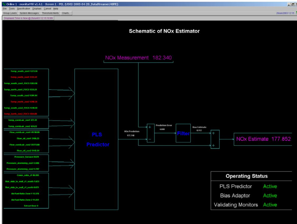
Figure 2: NOx on-line prediction schematic
