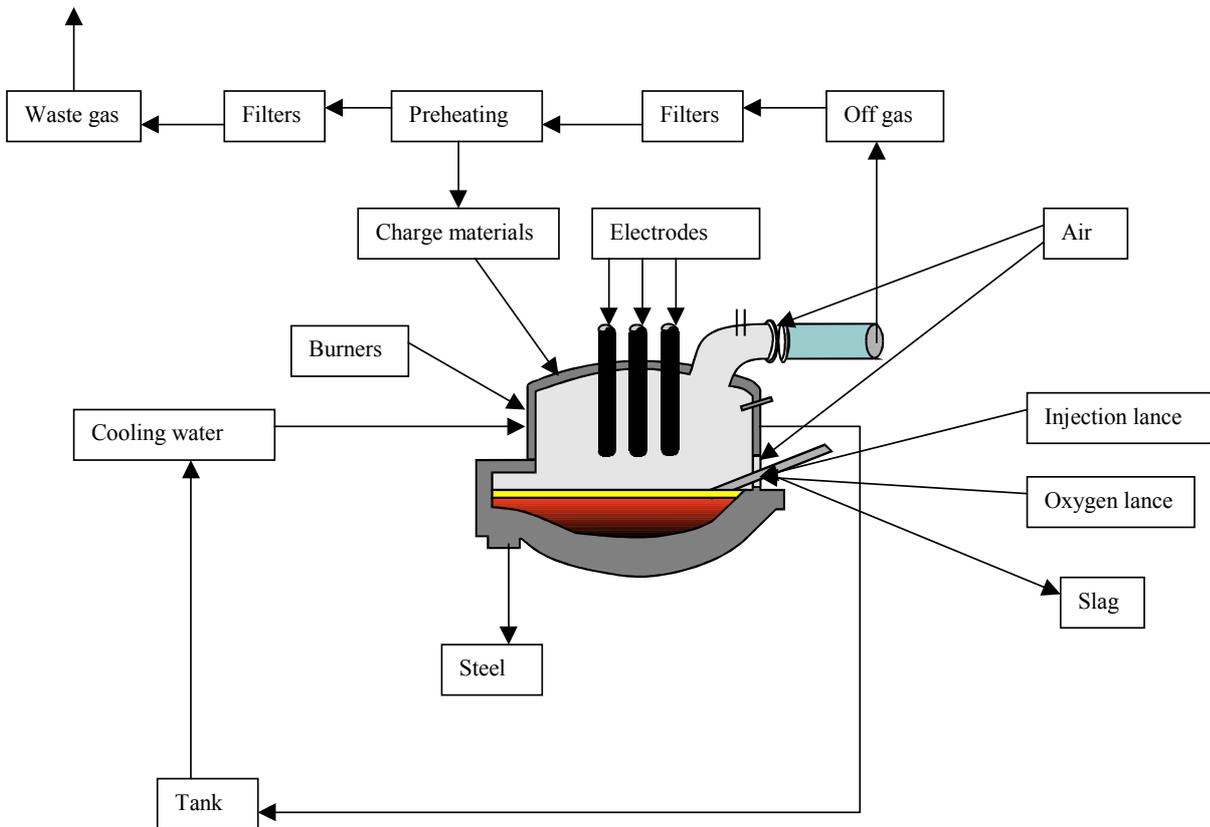
Figure 3b: Material Flow in an EAF
