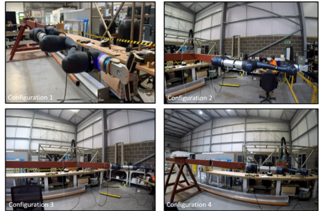
Fig. 1: Photographs of the 4 boom configurations (Configuration 1: Full-length boom with 180-degree hinge angle; Configuration 2: Full-length boom with 90-degree hinge angle; Configuration 3: Full-length boom with 45-degree hinge angle; Configuration 4: Half-length boom with 180-degree hinge angle).
