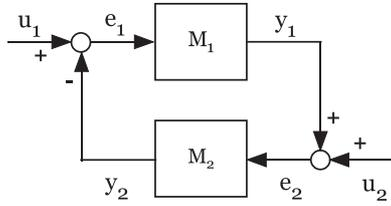
Fig. 4. Feedback interconnection of  $M_1$  and  $M_2$ .
