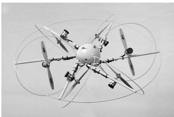
a) Hexrotor prototype. Rotor diameter 38cm, overall vehicle mass 5.5kg, hover duration 5 minutes
