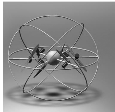
b) CAD illustration of a hexrotor vehicle in a rolling frame
