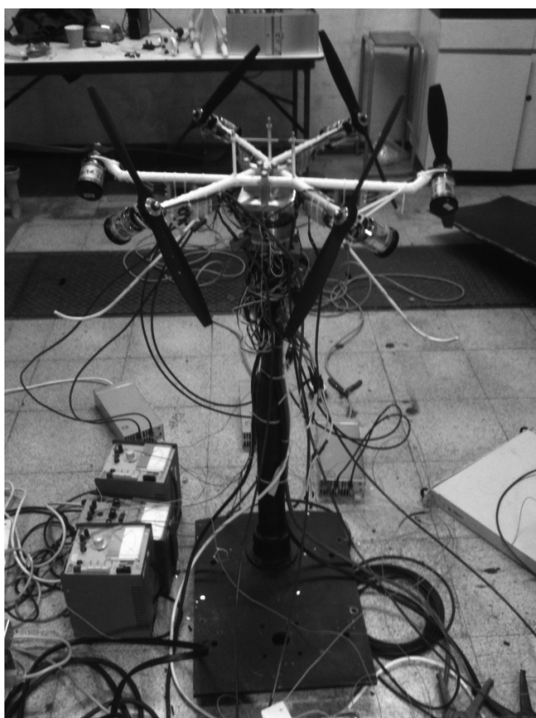
Fig. 12 Experimental setup for thrust and torque measurements.
