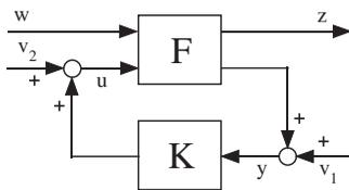
Figure 5. Internal stability of  $F_1(F, K)$ .
