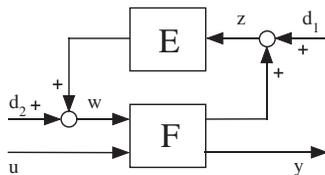
Figure A1. Mapping of  $(d'_2 \ d'_1 \ u')'$  to  $(w' \ z' \ y)'$ .
