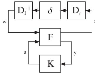
Figure 8. Internal stability of LTI system.
