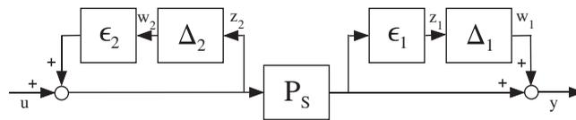
Figure 16. Open-loop shaped plant with uncertainty.
