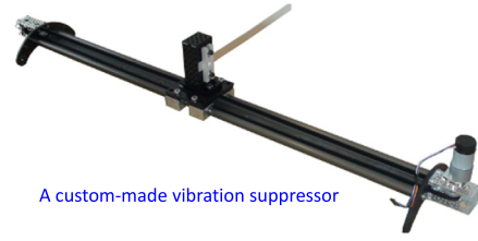
Fig. 2. A custom-made vibration suppressor for testing the NI-based IMC synthesis algorithms.
