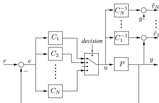
Fig. 2. An Adaptive Control Setup—Unfalsified Approach: Forward-path Controller Implementation
