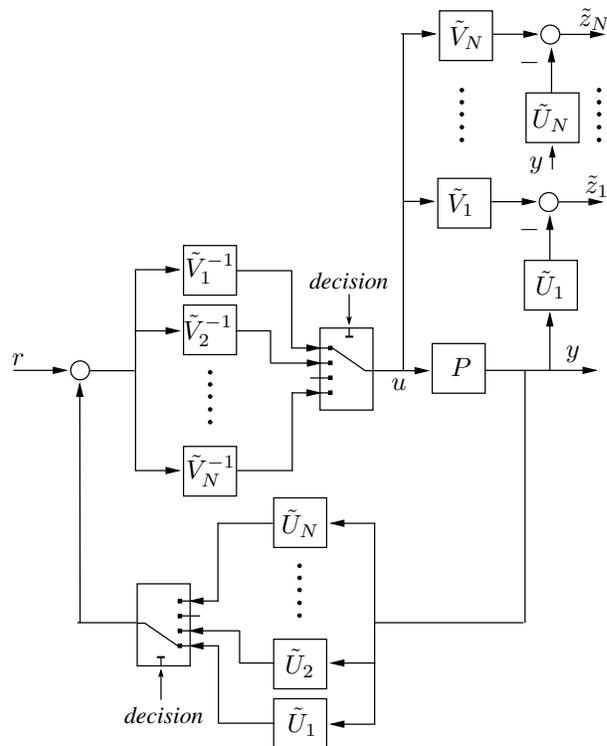
Fig. 6. Proposed Unfalsified Adaptive Control Setup
