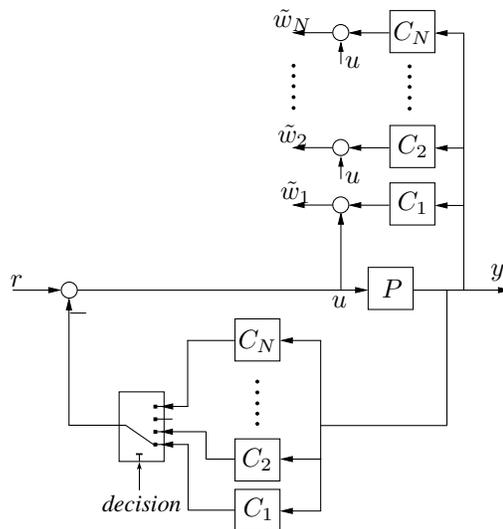
Fig. 3. Feedback-path Controller Implementation
