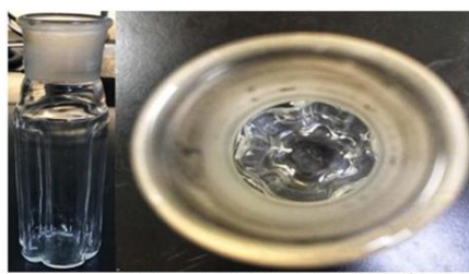
The six-baffled homemade glass vessel simulating Mozafari's glass bottle of 50 mL capacity.
