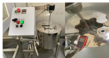
The six-baffled pilot scale tank of 13 L capacity.
