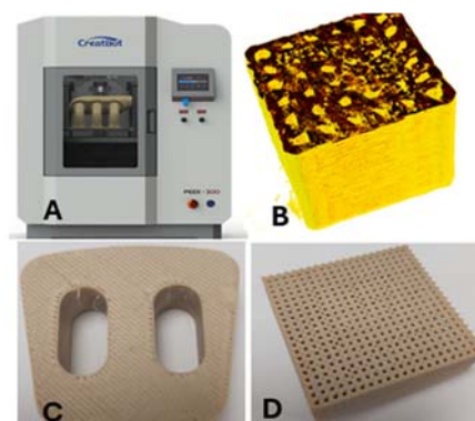
Figure 1 A) CreatBot printer B) MicroCT scan C) 3D printed spinal fusion device D) Basic Lattice
