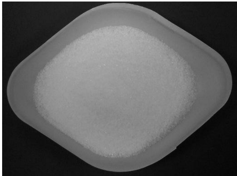
Figure 4.3 Shore Pac - PHPA polymer granules.
