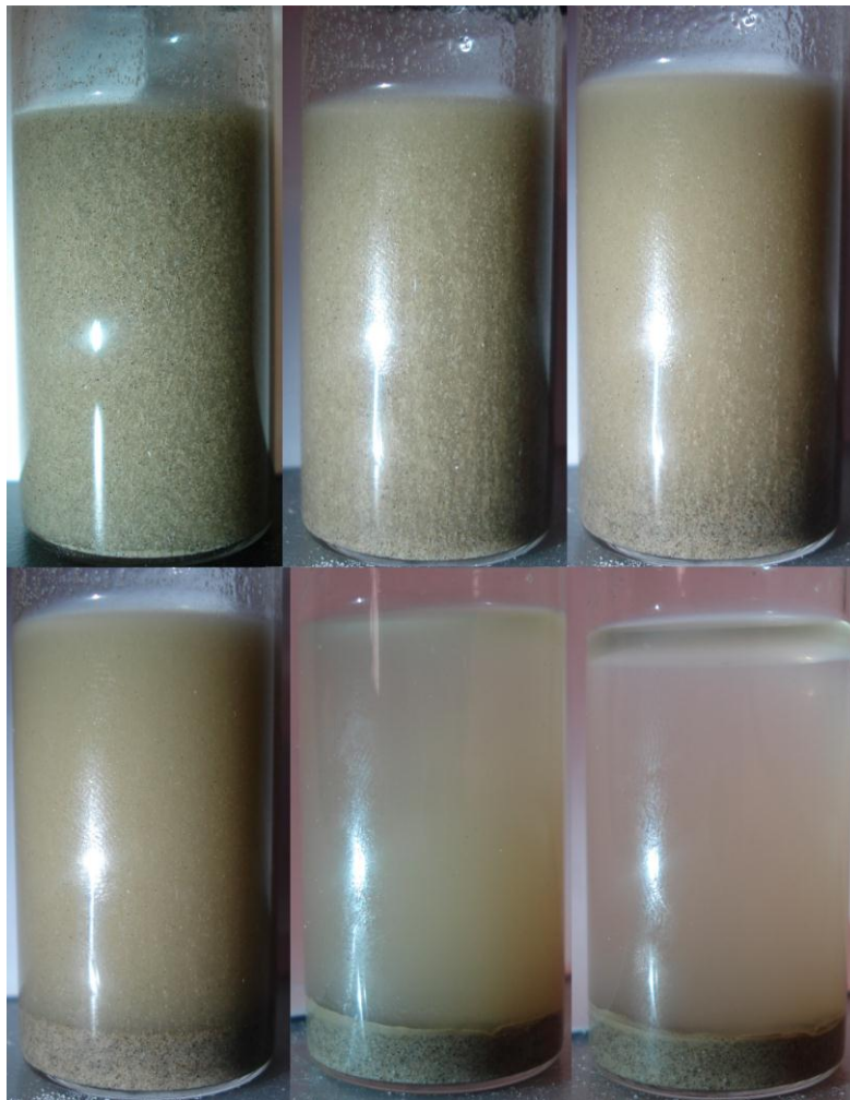
Figure 5.2 Sedimentation stages in a 5% suspension in a 0.2 g/L polymer. From left to right; top row: start, 30 seconds, 1 minute; bottom row: 10 minutes, 12 hours, 24 hours.
